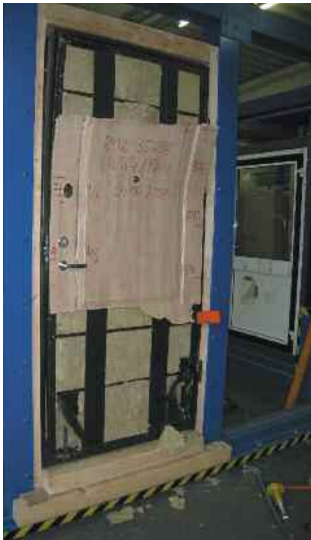
External opening door test
