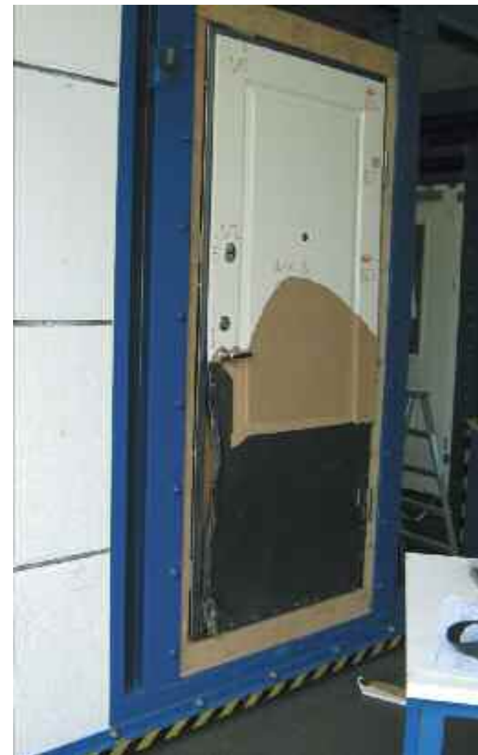
External opening door test
