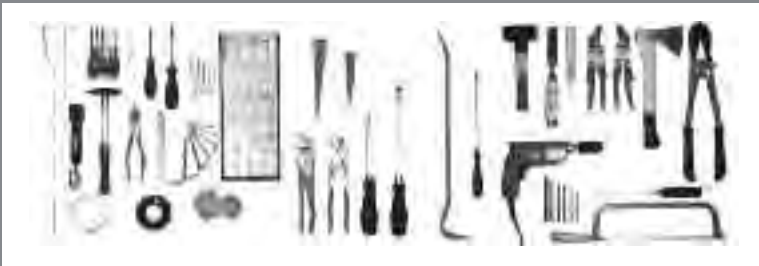
The tools used to test doors to burglary resistance class 4 (WK4) by EN 1627:2011.
